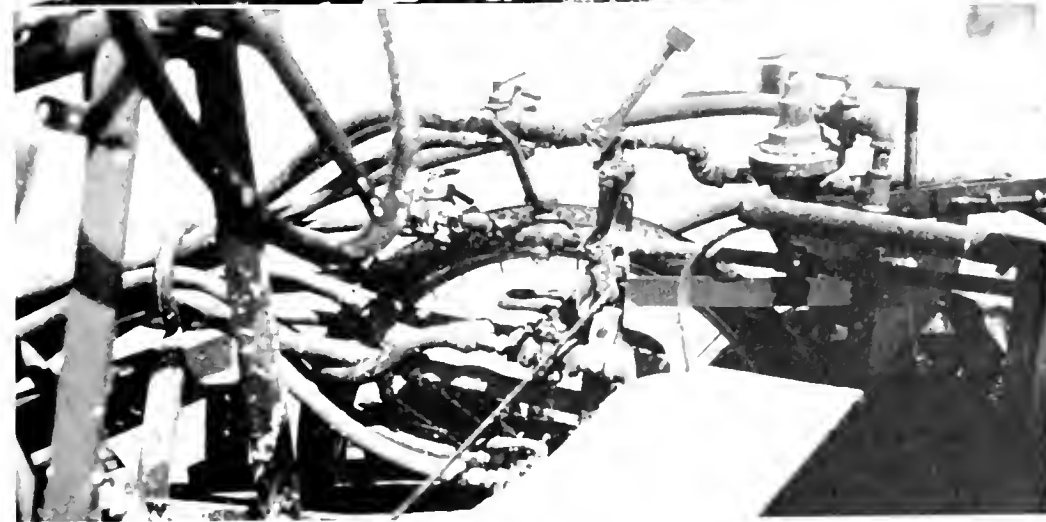
Top—Bicycle wheel operates attached cylindrical interrupter valve. Center—Rear view showing bead applicator mechanism. Bottom—Paint and air controls to spray guns
